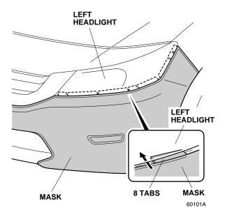
8. Pull the mask back toward the fenderwell, smooth out any wrinkles, and then snap the mask onto the snap-screw. Repeat on the right side.
