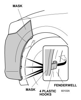
10. Attach four hooks to the inside edge of the front lower grille.
