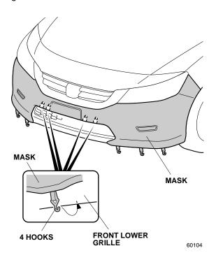
11. Attach three hooks to the hole of the under the front bumper. Repeat on the right side.
